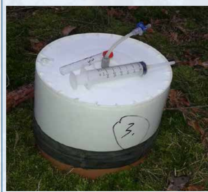
Measuring chamber (n=5/plot) (photo: M. Grüning)
